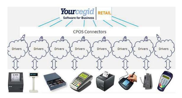
Instead of exchanging directly with each device, the POS terminal communicates with a generic multidevice connector called CPOS.
